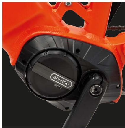
Bafang M510 36V 250W 95Nm motor, central
