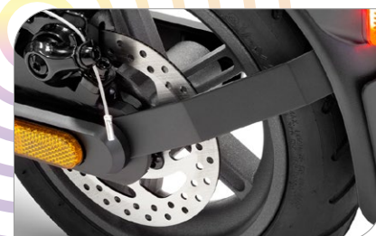
Front e-brake, rear disc brake, with 2 levers
